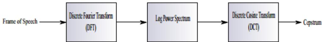
Figure 1. Block diagram of cepstrum calculation
