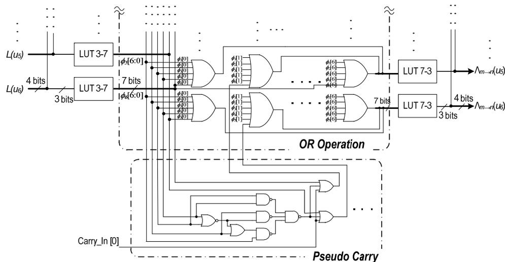
Figure 5. Proposed quasi binary weighting addition with pseudo-carry circuits.
