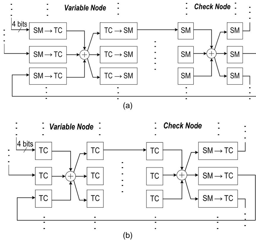
Figure 7. Datapath of variable node and check node message passing, (a) traditional architecture, (b) proposed TC based architecture.
