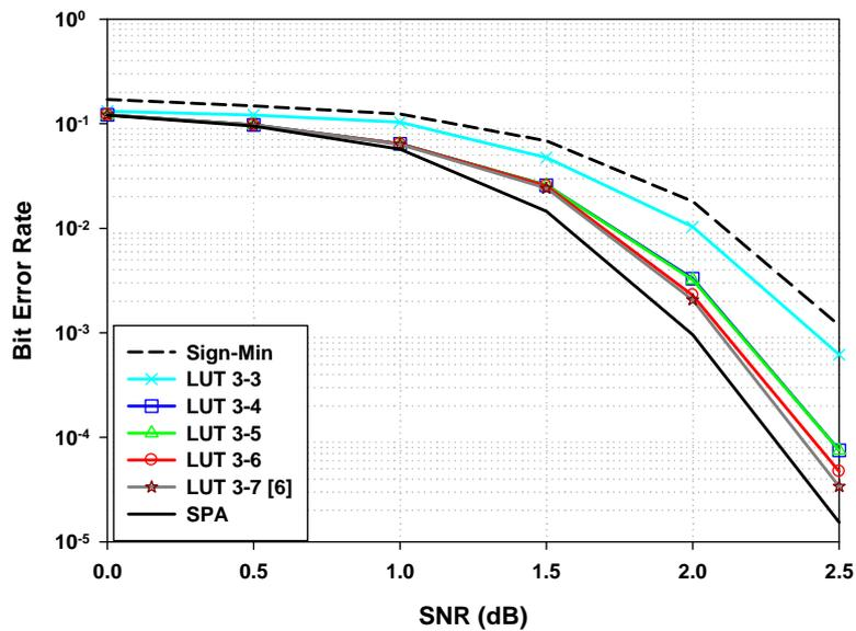
Figure 6. BER performance of different LUT for (1008, 504) LDPC code with eighty decoding iterations.
