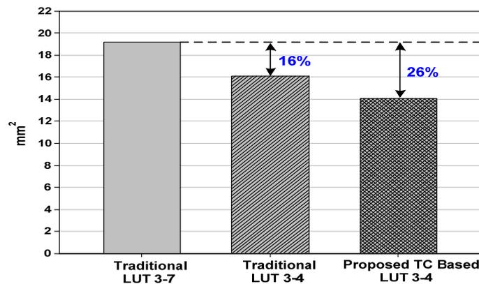
Figure 8. Hardware reductions with new TC based message passing architecture.
