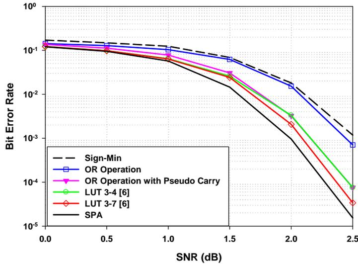
Figure 9. BER comparison for (1008, 504) LDPC code with eighty decoding iterations.
