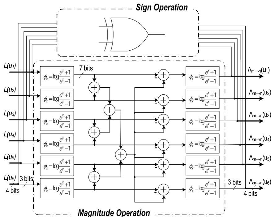
Figure 1. The traditional Log-SPA check node architecture.
