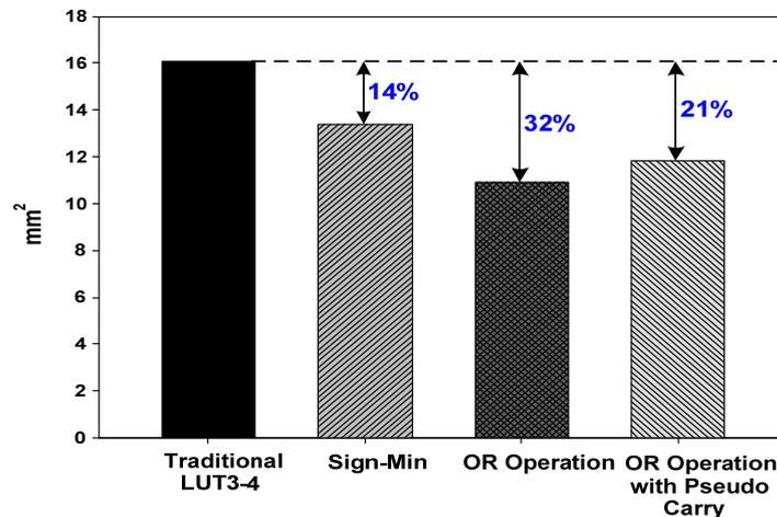
Figure 10. Area comparison of low hardware cost architectures using 0.18 $\mu$ m standard cell library.
