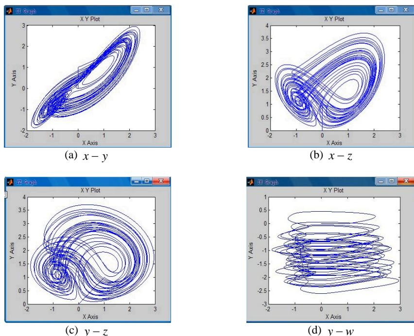
Figure 9. Plane phase diagram of digital hyper-chaotic system attractor ( $f_s = 1000\text{Hz}$ )
