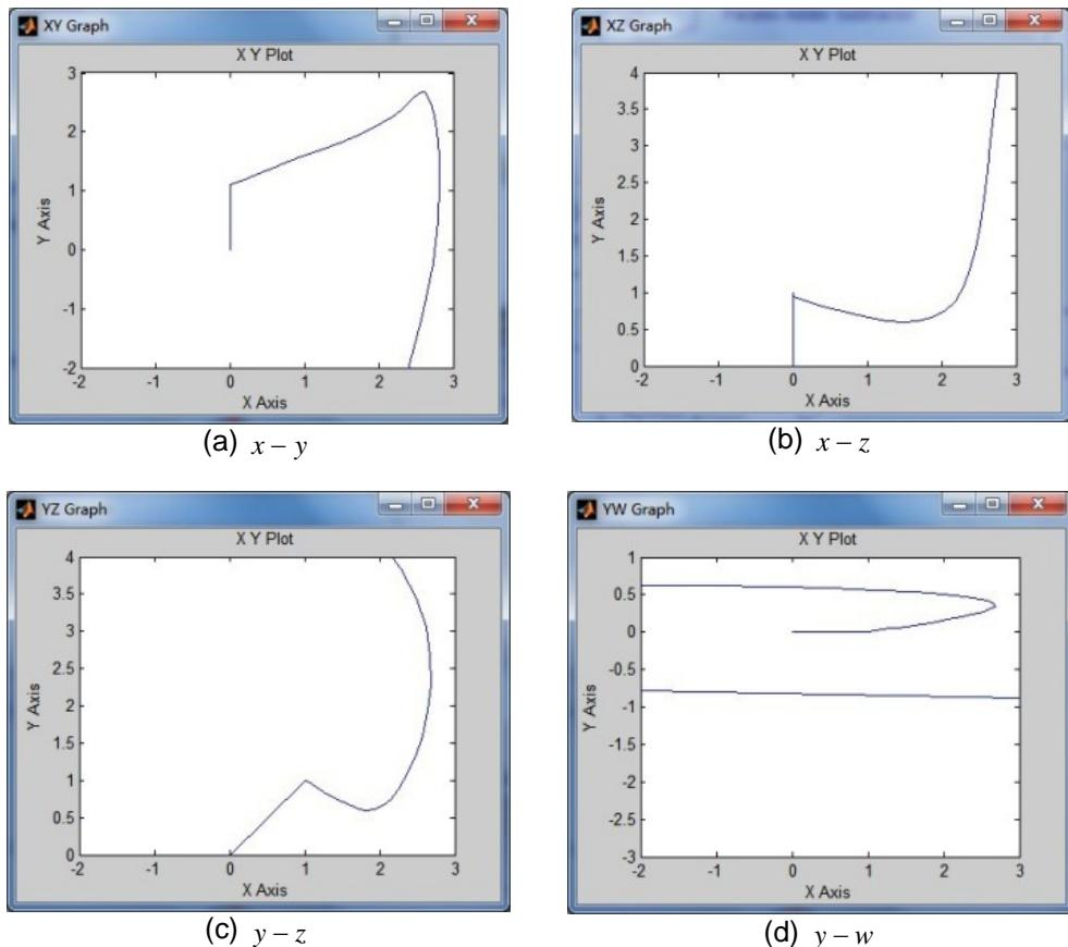
Figure 6. Plane phase diagram of digital hyper-chaotic system attractor ( $f_s = 50\text{Hz}$ )
