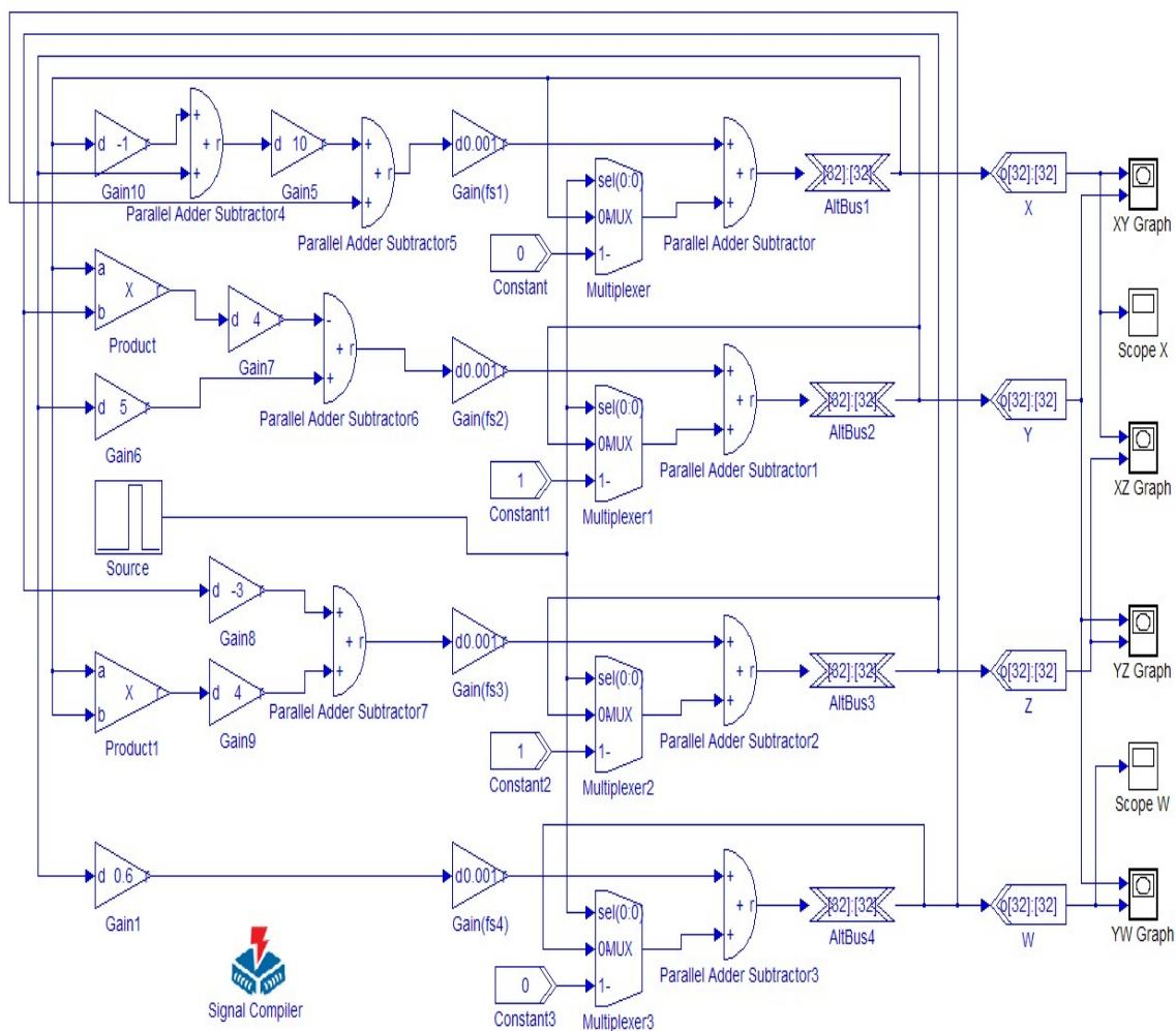
Figure 4. Digital circuit of hyperchaotic system based on DSP Builder
