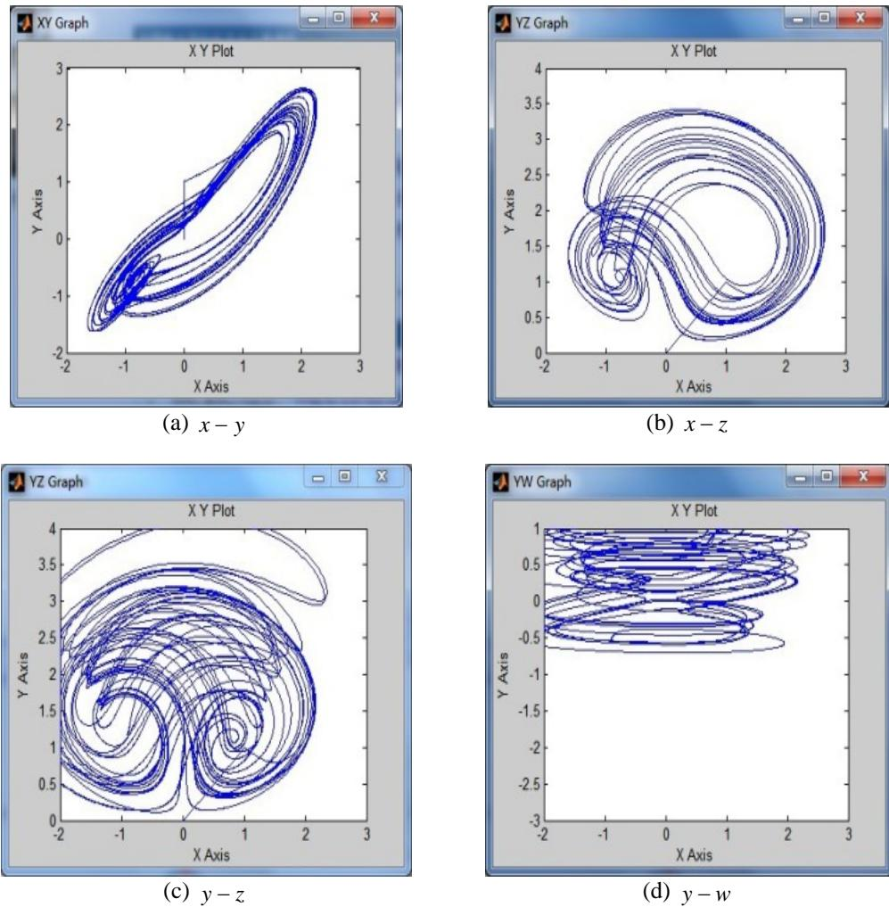
Figure 7. Plane phase diagram of digital hyper-chaotic system attractor ( $f_s = 250\text{Hz}$ )
