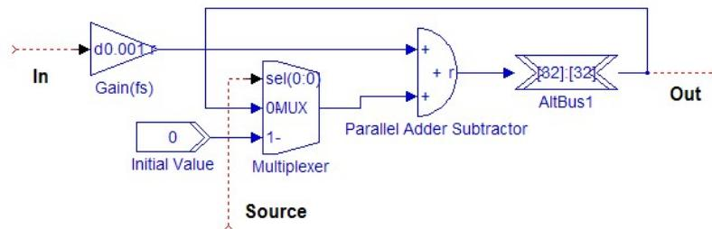
Figure 3. Digital integrator that can adjust the sampling frequency flexibly
