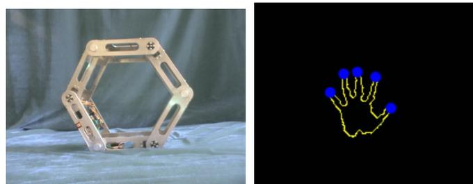
Figure 6. Recognition of gesture "all-extended" and the shape change of the hexagon robot
