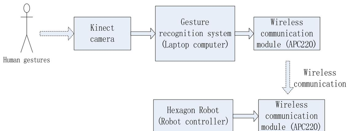
Figure 1. The system structure of the robot control system based on gesture recognition
