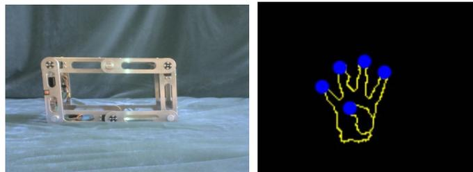
Figure 5. Recognition of gesture "four" and the shape change of the hexagon robot
