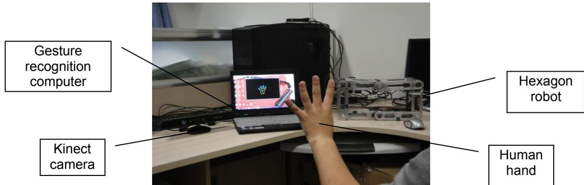
Figure 3. The gesture recognition system and the hexagon robot
