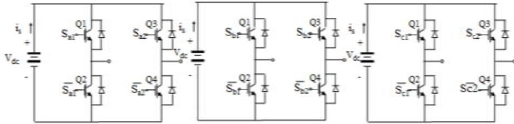
Figure 2. Three levels cascaded H-bridge inverter
