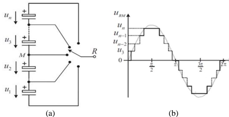
Figure 1. (a) Simplified circuit of a n-level converter, (b) generated output n-level voltage
