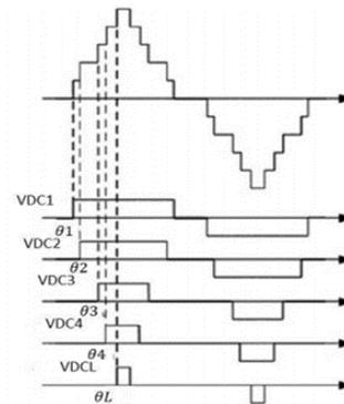
Figure 3. Staircase voltage waveform for single-phase three-level inverter [16]
