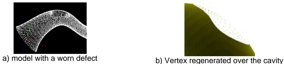
Figure 8. Vertex regeneration for a worn shaft
