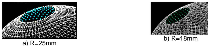
Figure 11. Regenerated Vertices on the worn area of a sphere with R=25mm,18mm
