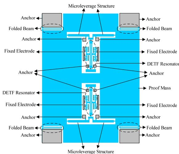
Figure 1. Structure diagram of the micro-mechanical silicon resonant accelerometer.
