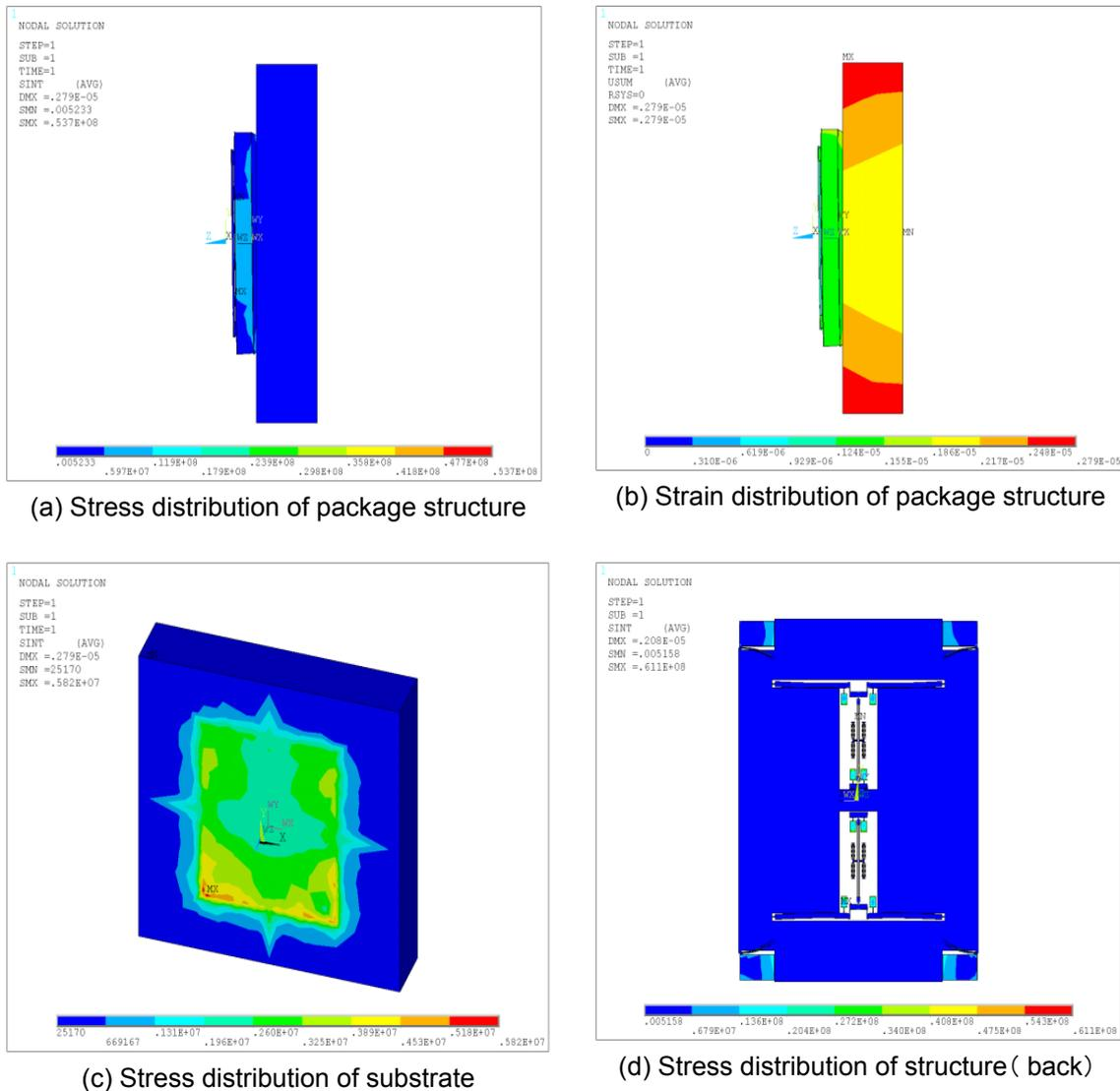
Figure 7. Stress and strain distribution of package structure
