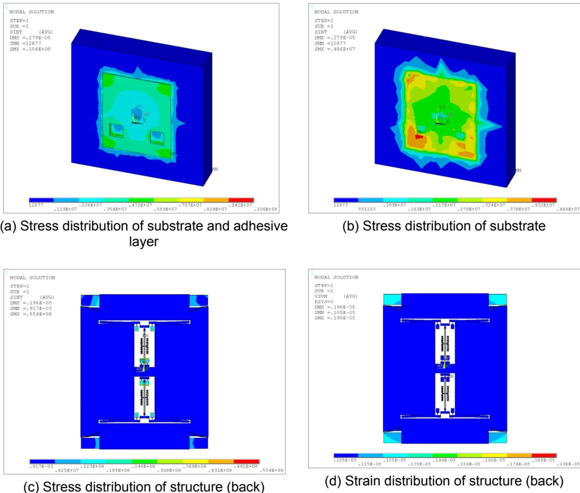
Figure 10. Stress and strain distribution of package structure (asymmetrical defects)
