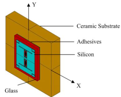
Figure 2. 3-D simulation model of the packaged micromechanical silicon resonant accelerometer.
