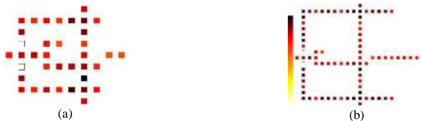
Figure 9. Energy dissipation map for proposed (a) comparator (without clocking) (b) comparator (with clocking) at 1.5 E_k
