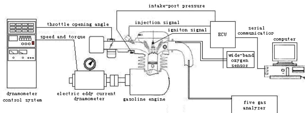
Figure1. Diagram of Experimental System
