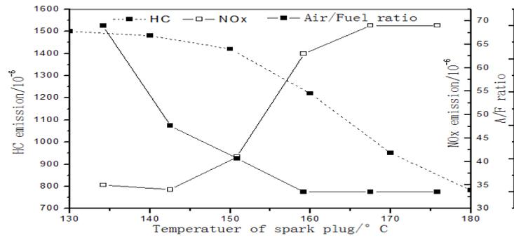
Figure 4. Trend of HC and NOx With Increase of Temperature
