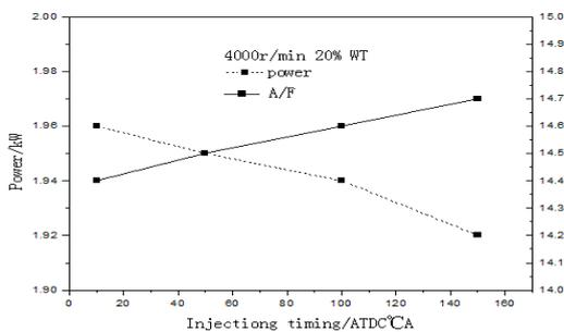
Figure 5. Engine Power And A/F Ratio Changed With Injection Timing
