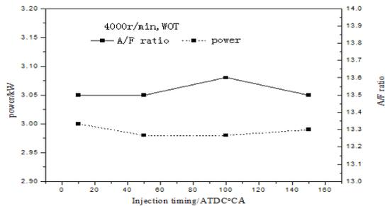
Figure 7. Engine Power And A/F Ratio Changed With Injection Timing
