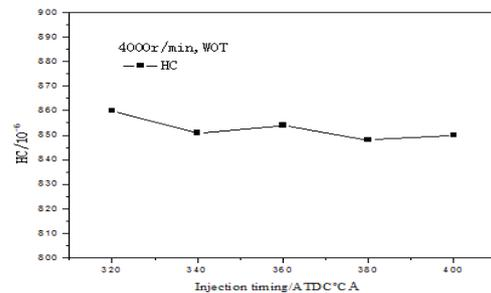
Figure 12. HC emission changed with injection timing
