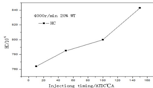
Figure 6. HC Emission Changed With Injection Timing
