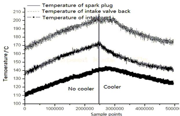
Figure 3. Trend of Temperature At Different Measure Points
