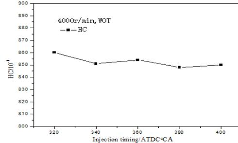
Figure 8. HC Emission Changed With Injection Timing
