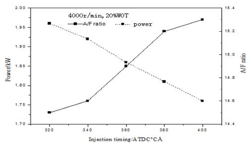
Figure 9. Engine Power And A/F Ratio Changed With Injection Timing
