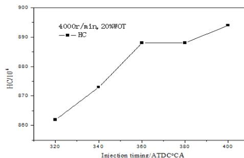
Figure 10. HC Emission Changed With Injection Timing
