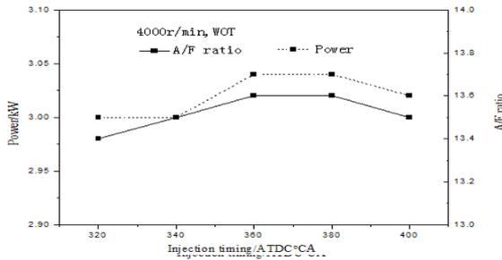
Figure 11. Engine power and A/F ratio changed with injection timing
