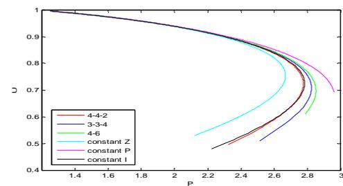
Figure 6. P-V Curve of Mode 3
