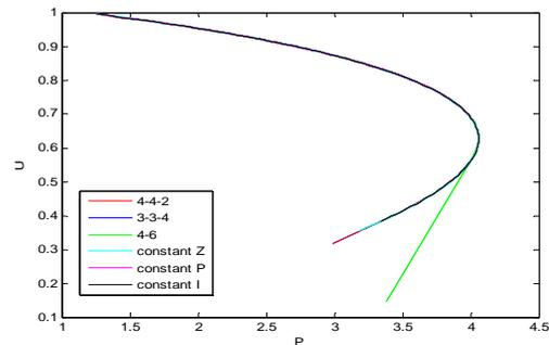
Figure 4. P-V Curve of Mode 1
