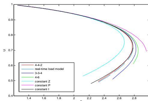
Figure 7: P-V Curve of 9-node System with Real-time Load Model
