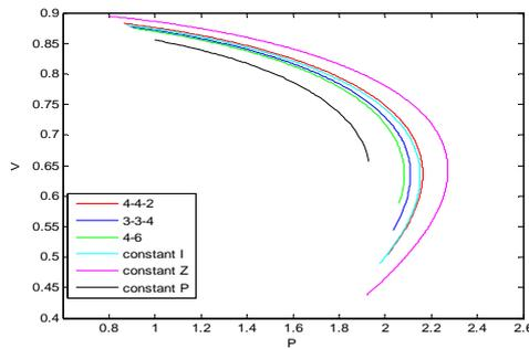
Figure 2. P-V Curves of 2-node System
