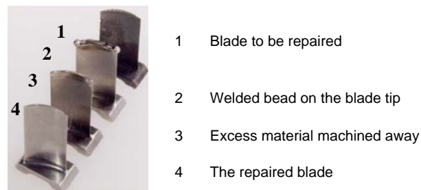
Figure 7. Repair of a straight blade tip (RB199 HPC vanes, MTU)
