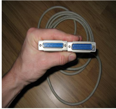
Figure 5. Parallel port with 25 pin out
