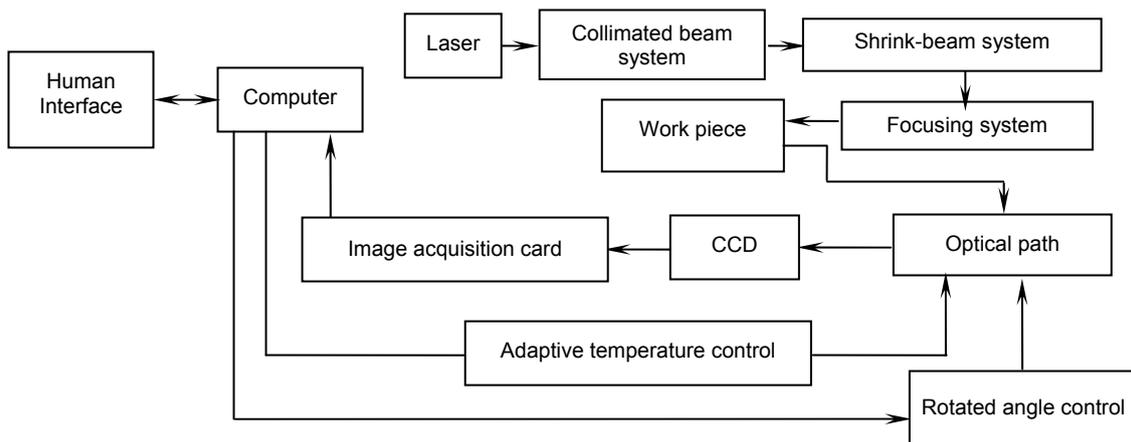
Figure 2. Block diagram of Conoscopic Holography system
