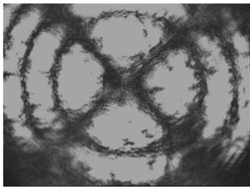
Figure 3. Normal incident conoscopic holography
