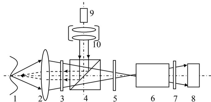
1-object; 2-objct lens; 3, 5- $\lambda/4$  wave plate; 4-polarization spectroscopy, 6-uniaxial crystal, 7-polarizing disc, 8-CCD, 9-laser, 10-collimated beam system
