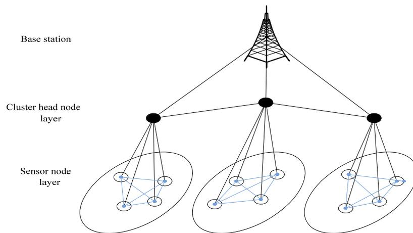
Figure 1. Hierarchical wireless sensor network model
