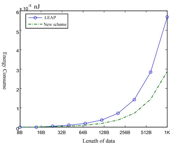
Figure 9. Node energy consumption in the key establishment phase
