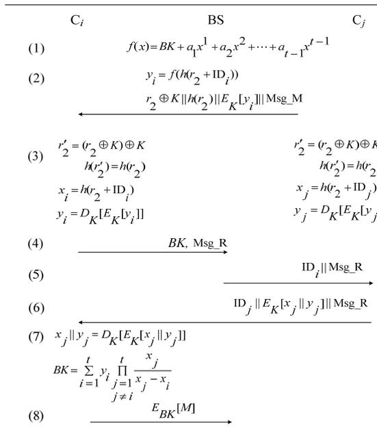
Figure 4. Master key distribution and reconstruction process
