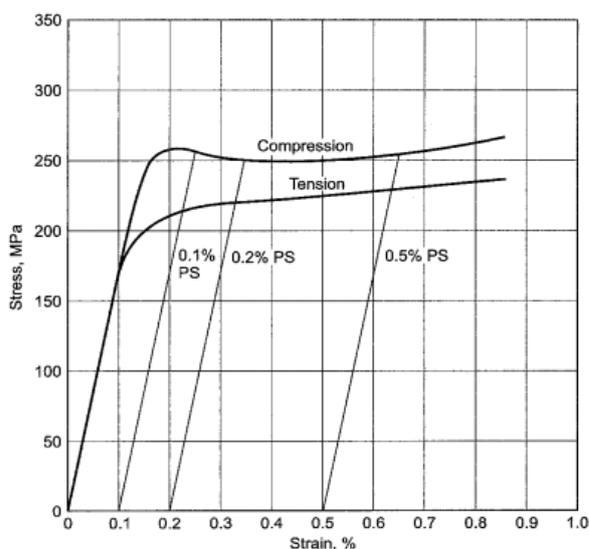
Figure 3. The stress-strain curve of KTH330-08 malleable iron
