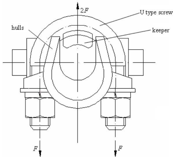
Figure 1. The connection schematic diagram of U type screw and clamp hulls
