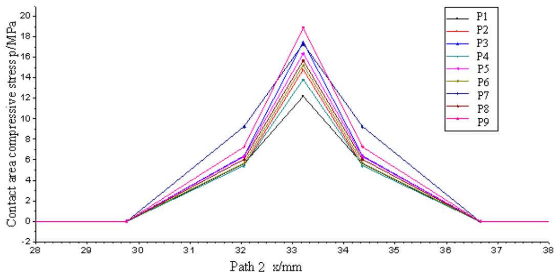
Figure 8. Distribution of contact stress along path 2
