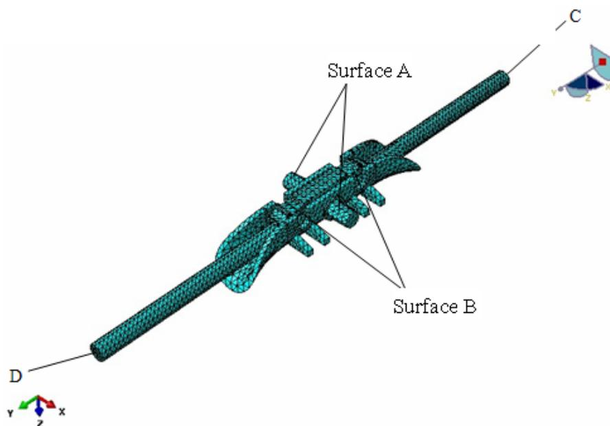
Figure 2. The finite element model of the contact between conductor and clamp
