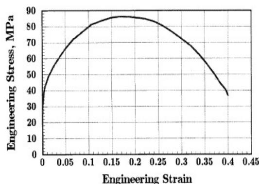
Figure 4. The stress-strain curve of the aluminum wire materials
