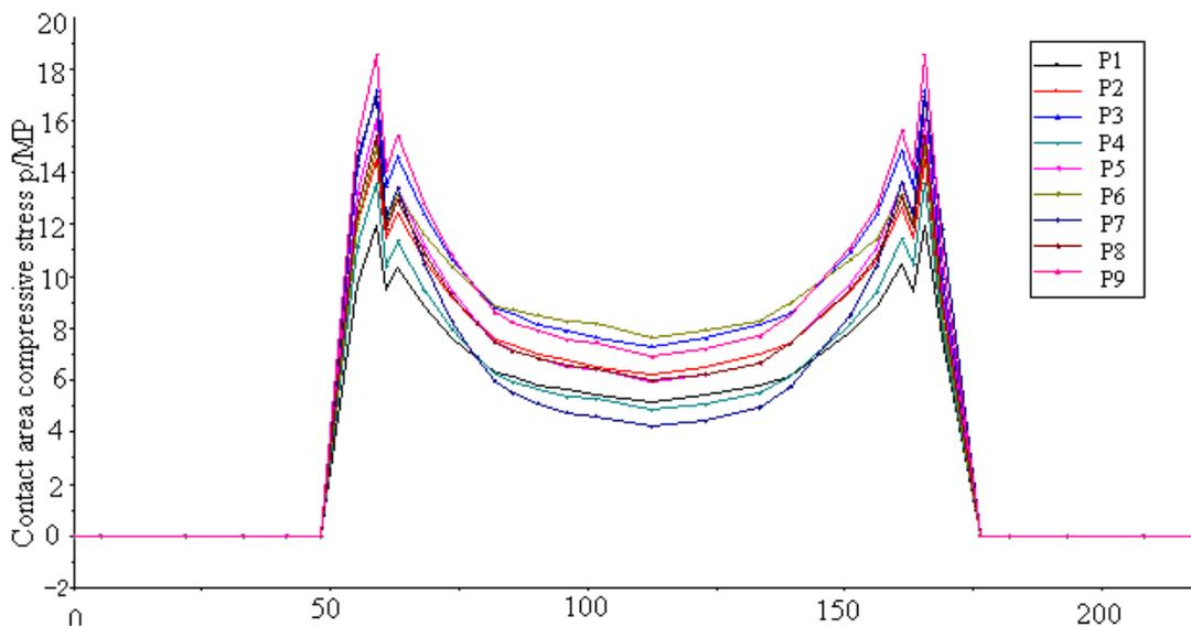
Figure 7. Distribution of contact stress along the path 1
