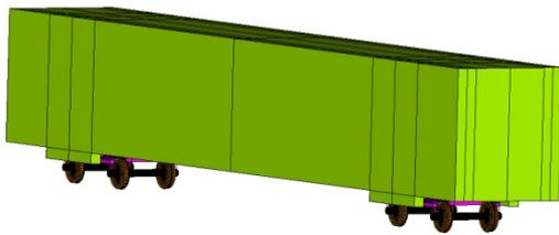
Figure 5. Vehicle finite element model
