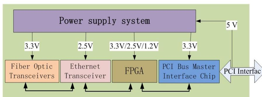
Figure 2. Hardware Structure of Data Transmission System
