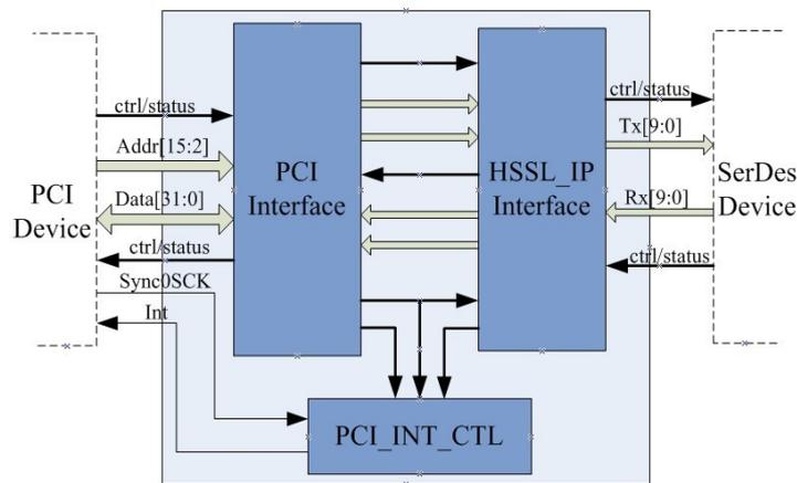
Figure 3. The interface diagram of Data Transmission System
