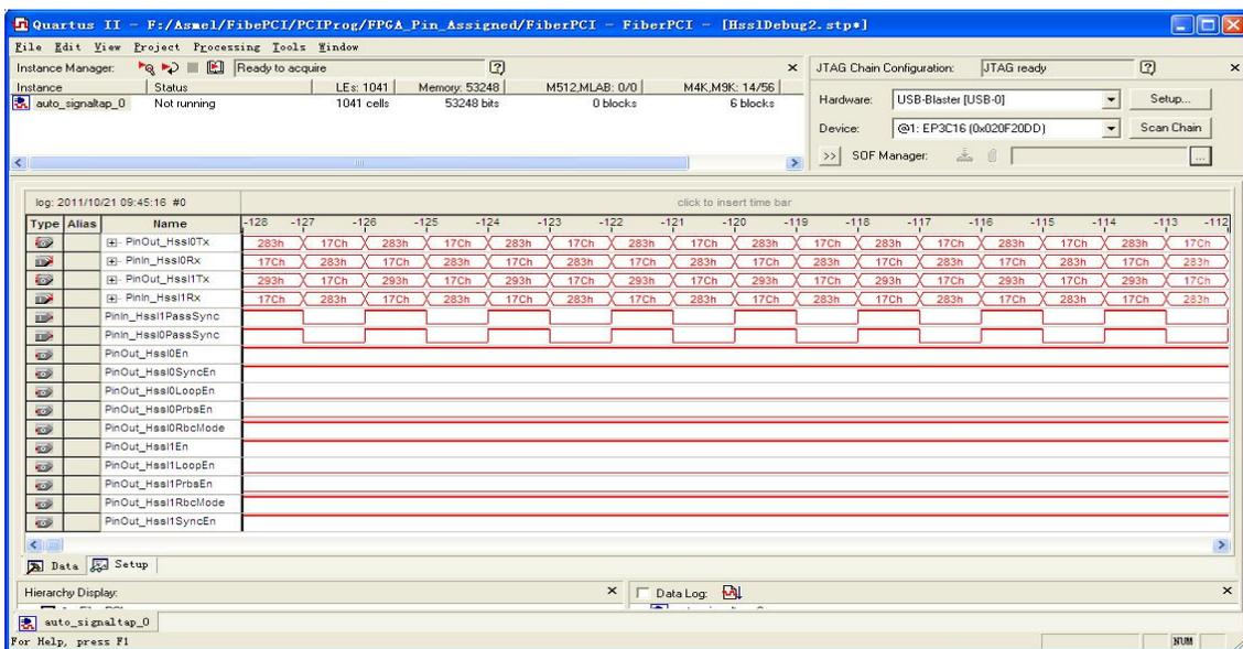
Figure 9. The Signal Tap II logic analysis
