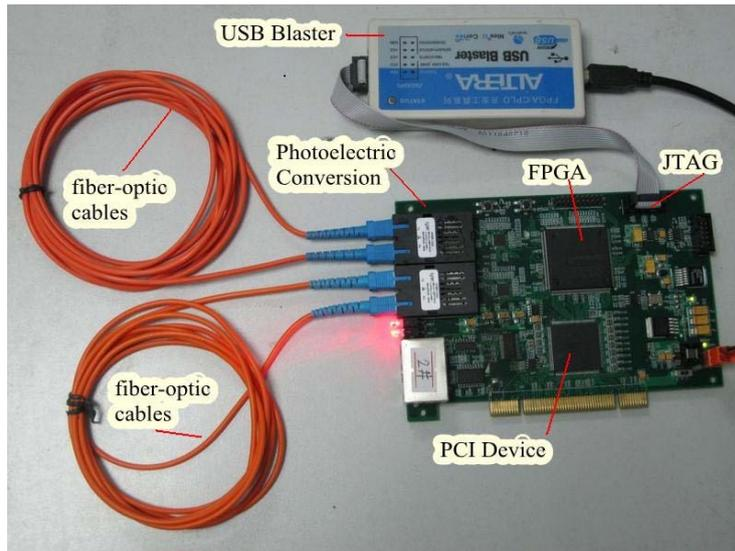
Figure 8. The test of the fiber optic interface
