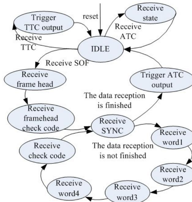
Figure 7. The state transition of the receiver module
