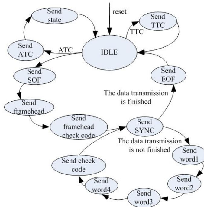
Figure 6. The state transition of the transmission module
