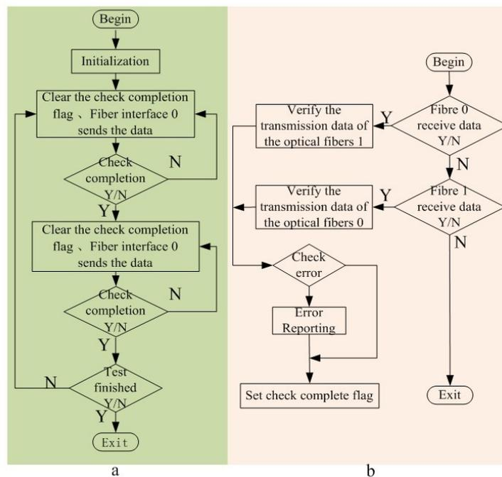
Figure 11. Test process of the Data Transmission System
