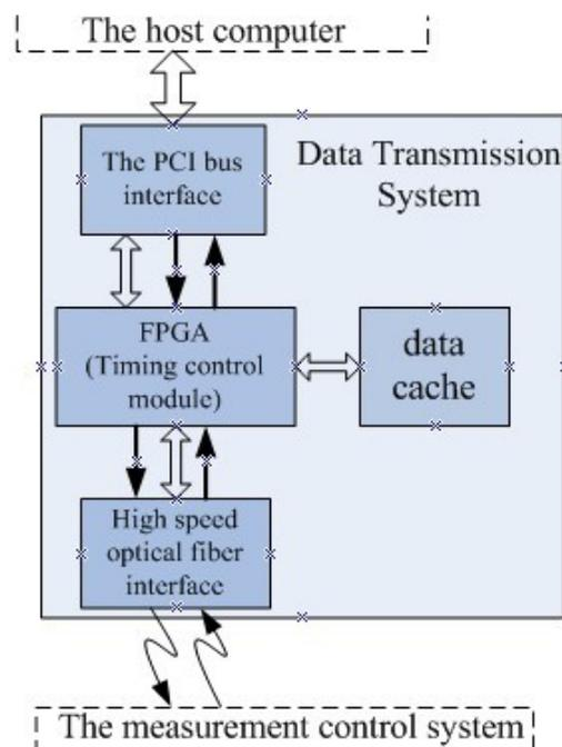
Figure 1. Architecture of Data Transmission System
