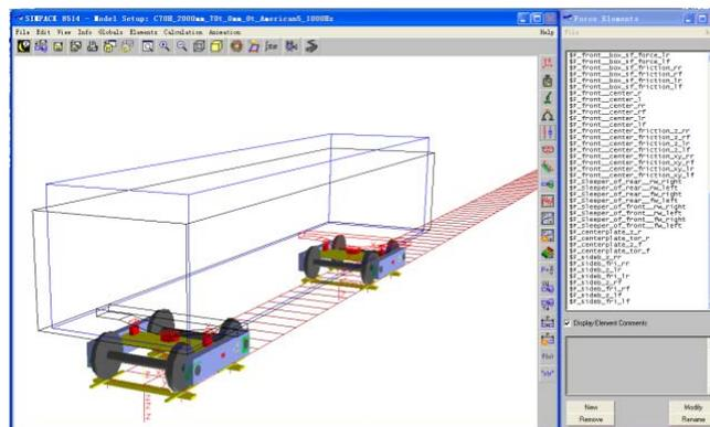
Figure 5. Virtual gondola car system model interface
