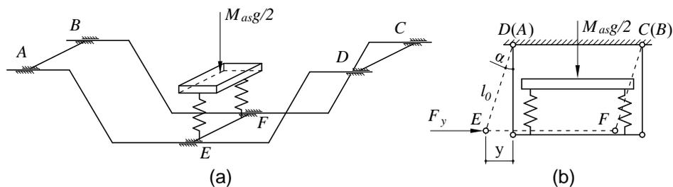
Figure 3. Diagram of side frames for swing motion truck
