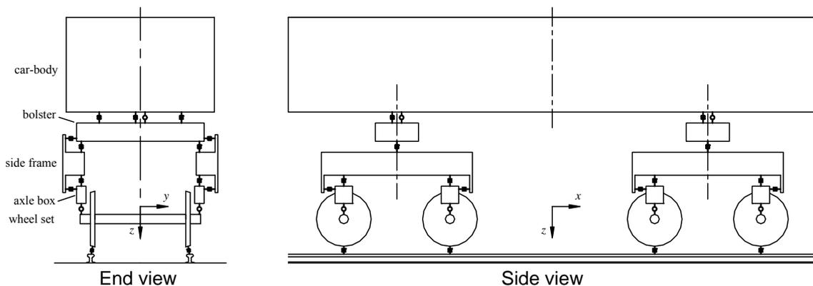
Figure 2. C70H gondola car system topology graph
