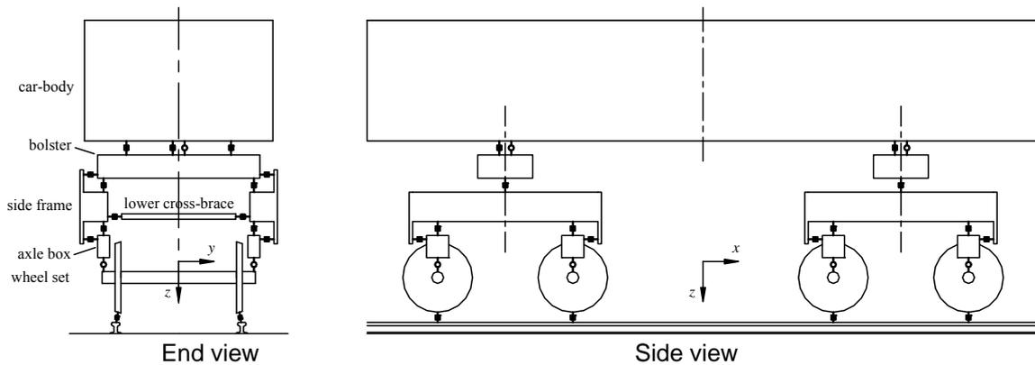
Figure 1. C70 gondola car system topology graph
