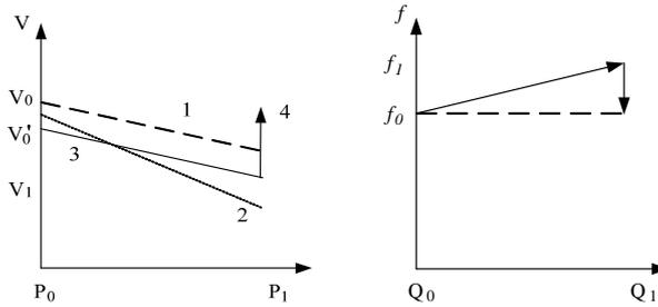
Figure 2. Control diagram of virtual-impedance-droop
