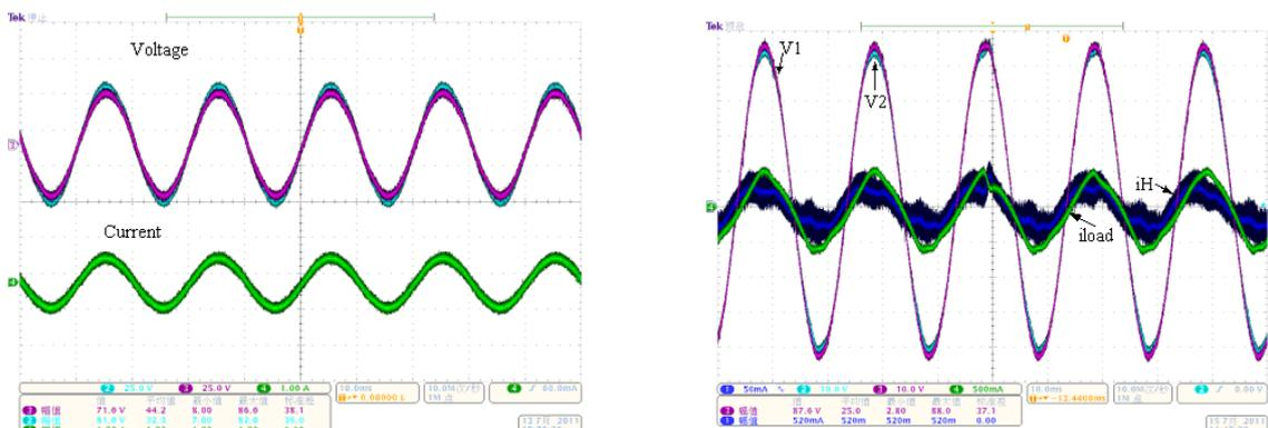
(a) Inverter's output voltage/current during parallel (b) output voltage/current & circulating current
