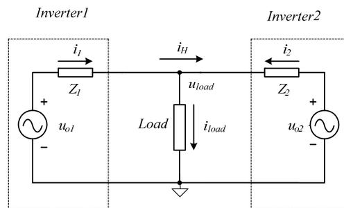
Figure 6. Two inverters in parallel
