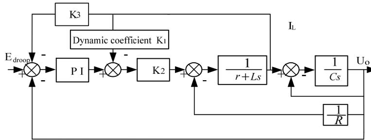
Figure 3. Controller module of virtual impedance
