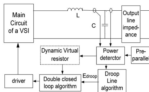
Figure 1. Droop control schematic diagram of a VSI
