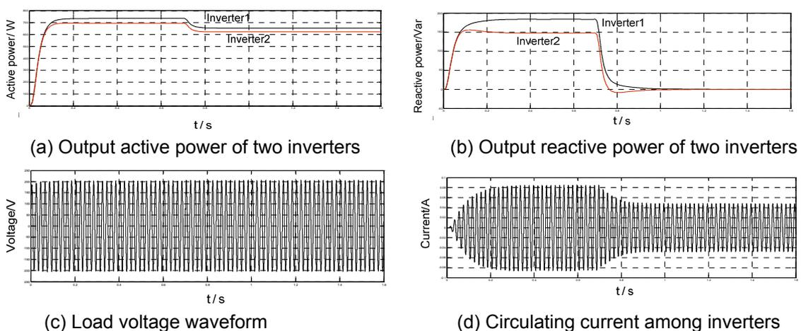
Figure 7. Dynamic state waveform of dynamic virtual resistance and droop control simulation
