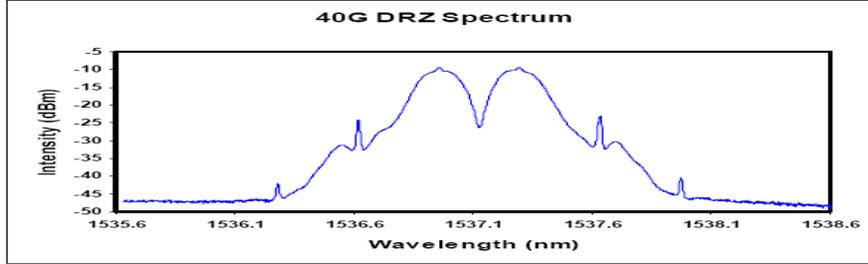
Figure 7. DRZ 40G DWDM OTU Typical Spectrum
