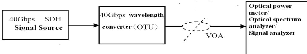
Figure 5. Configuration Diagram of 40 G OTU Performance Test
