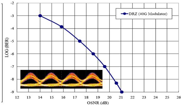
Figure 10. 40G DWDM 1600km long-fiber Transmission BER and OSNR Curve
