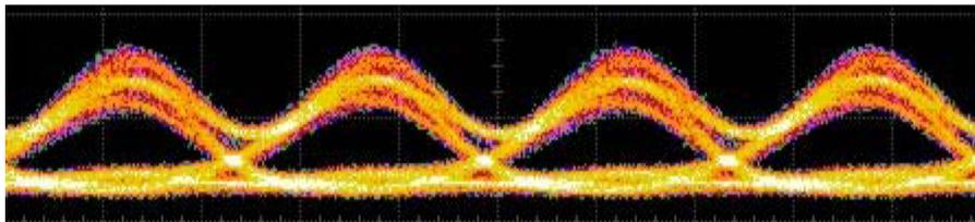
Figure 8. DRZ 40G DWDM OTU Typical Eye Diagram
