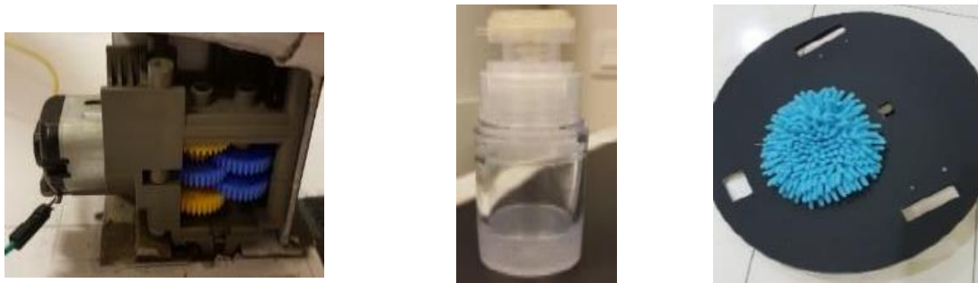
(a) Tamiya's gearbox packs with DC motor (b) Water spray bottle (c) Position of wiping material
