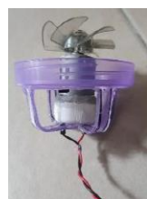
(a) Motor for vacuum unit
