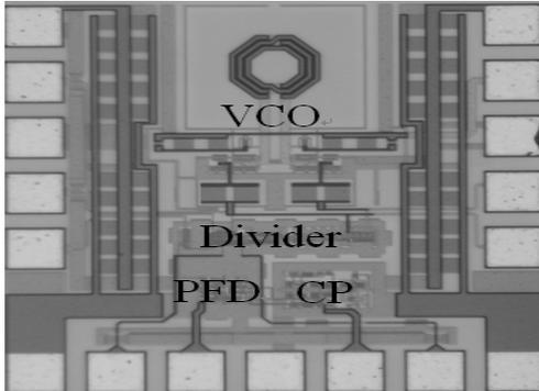
Figure 11. Microphotograph of The Frequency Synthesizer
