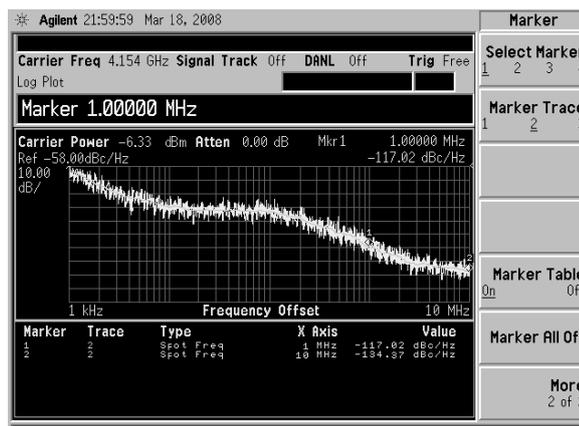
Figure 15. Measured Phase Noise of Frequency Synthesizer in The Locked State
