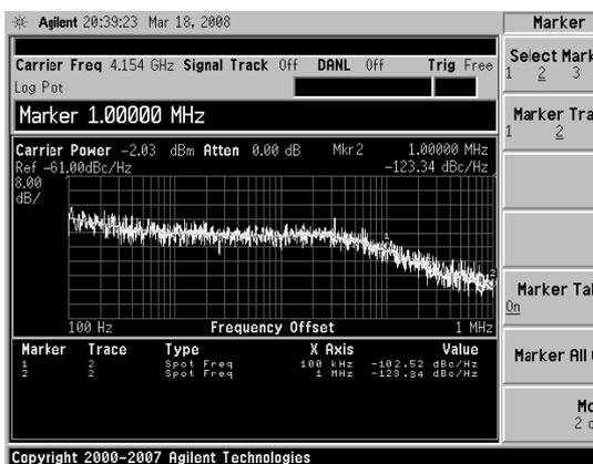
Figure 13. Measured Phase Noise of VCO
