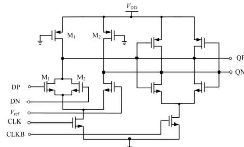
Figure 8. D-latch Architecture With OR Input
