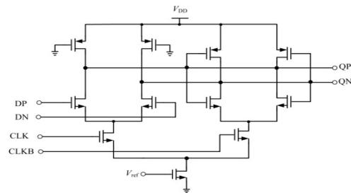
Figure 6. Circuit Schematic of The Latch Voltage
