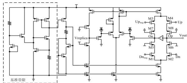
Figure 10. Circuit Schematic of Charge Pump
