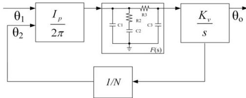
Figure 3. Linear Model for The CPLL Type Frequency Synthesizer
