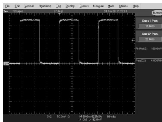
Figure 14. Waveform of Down-Scaler in The Locked State
