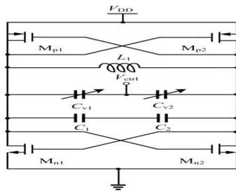
Figure 5. Circuit Schematic of The VCO
