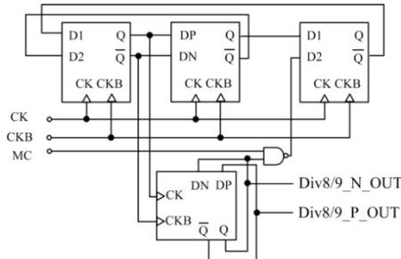
Figure 7. Block Diagram of The Dual-Modulus Divider-by-8/9 Prescaler
