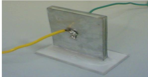
Figure 1. ER fluid sample container
