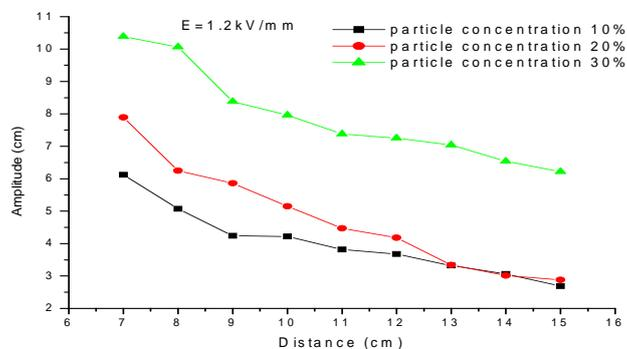
Figure 5. Sound amplitude varies with propagation distance and particle Concentration under the same electric field
