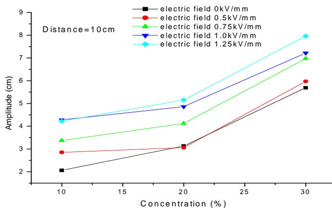
Figure 8. Sound amplitude varies with particle concentration and electric field at fixed distance
