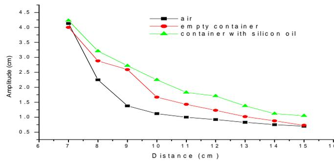
Figure 3. Sound amplitude varies with distance in different mediums
