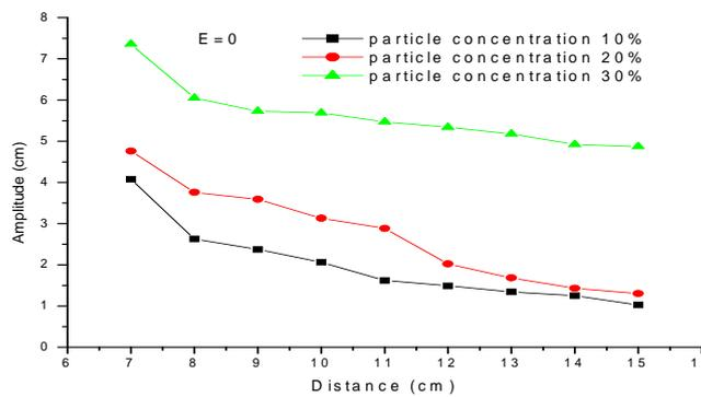
Figure 4. Sound amplitude varies with propagation distance and particle Concentration without electric field
