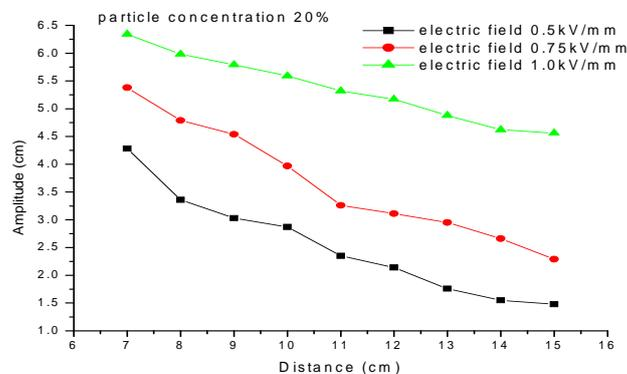
Figure 6. Sound amplitude varies with propagation distance and electric field at the same particle concentration
