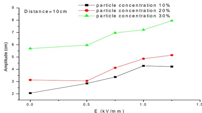
Figure 7. Sound amplitude varies with electric field and particle concentration at fixed distance
