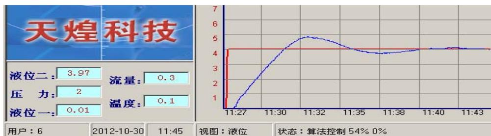
Figure 12. The experimental response curve of optimizational variable integral PID control(cm/min)
