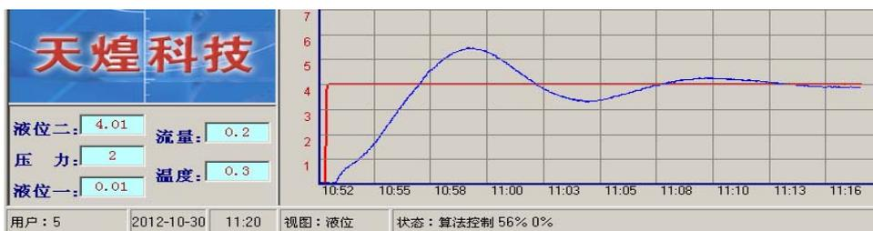
Figure 10. The experimental response curve traditional PID control(cm/min)
