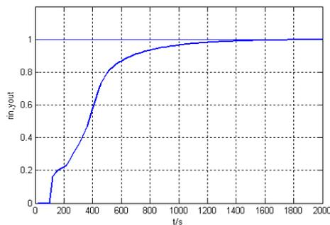
Figure 6. The step response curve of traditional variable integral PID control
