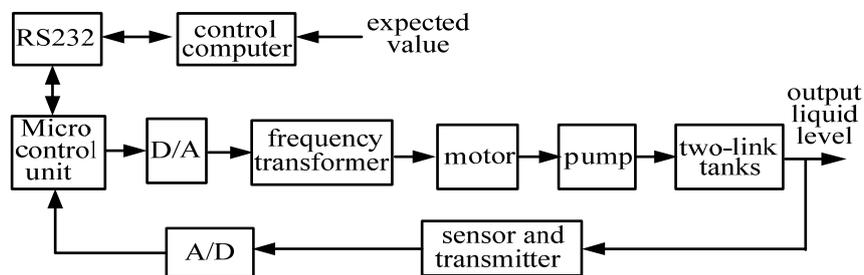
Figure 8. The liquid level control system block diagram of two-link tanks system
