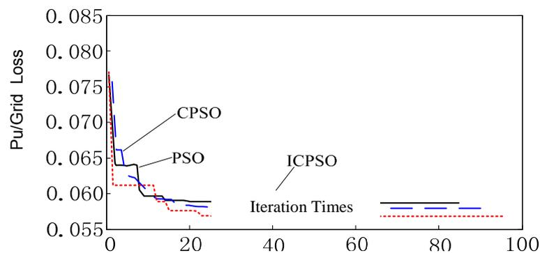
Figure 2. Convergence curves of PSO, CPSO and ICPSO algorithms
