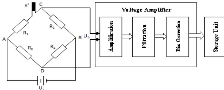
Figure 2. Schematic drawing of a strain measuring chain with an SLM strain gage
