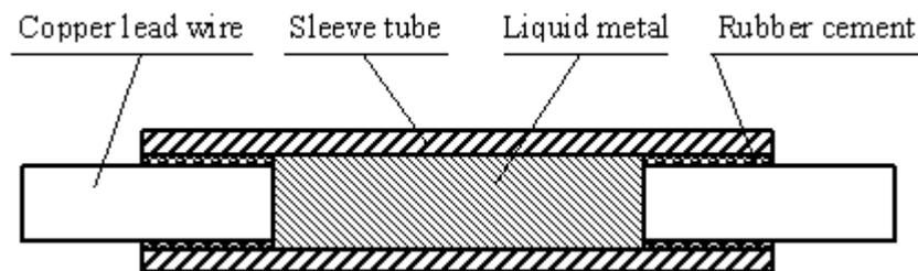
Figure 1. Scheme of the miniature strain gage of liquid metal
