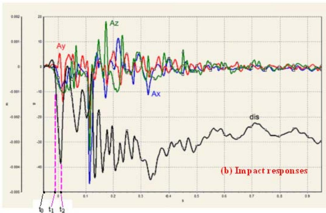
Figure 7. Impact responses of the PM during the rear-end crash (**Ax** and **Az**: head acceleration components which are mutually orthogonal in the sagittal plane; **Ay**: head acceleration component vertical to the sagittal plane. **dis**: neck tensile displacement; see online version for colours)
