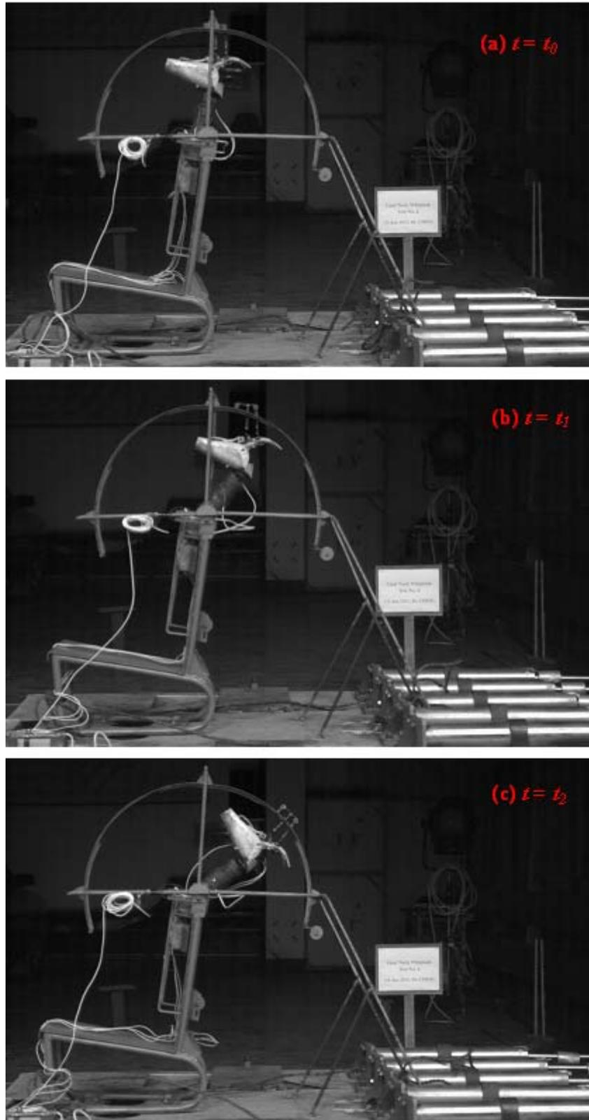
Figure 8. High-speed photo images of the PM during the rear-end crash (see online version for colours)
