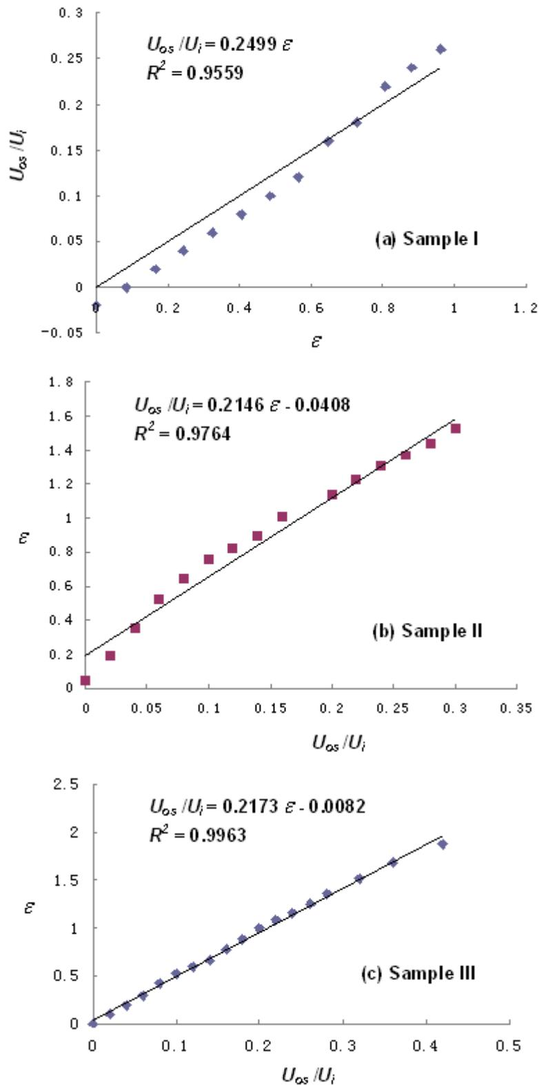
Figure 6. Calibration equation of Calibration curve of three strain gage samples
