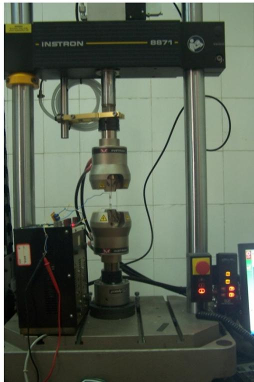
Figure 3. Calibration setup of Sample 1 (see online version for colours)
