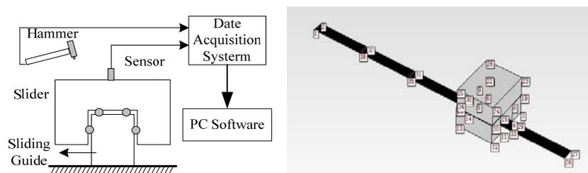
Figure 4. The schematic of experiment and measuring points
