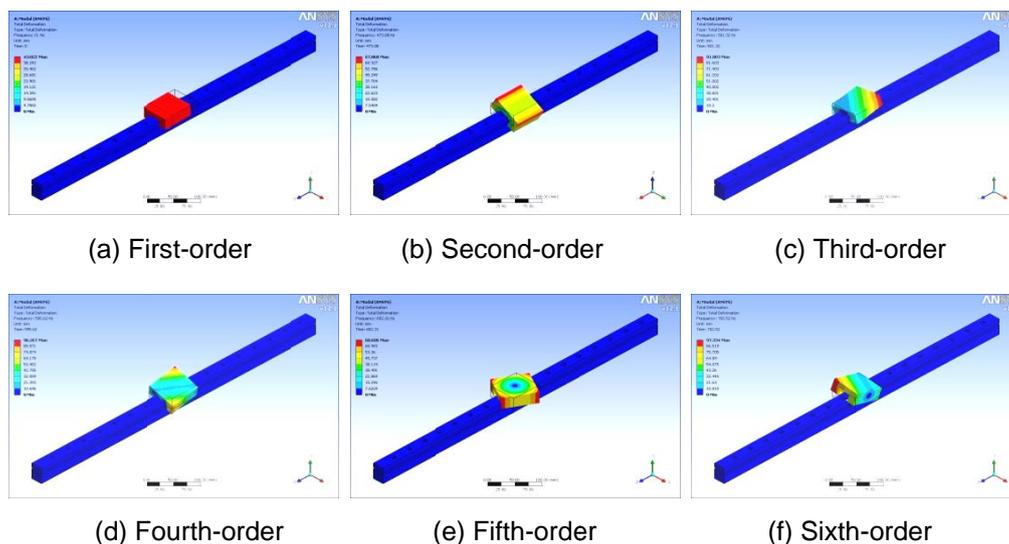
Figure 3. The first 6-order vibration modes on boundary condition 2
