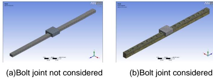
Figure 1. FEM of the guide with different situation
