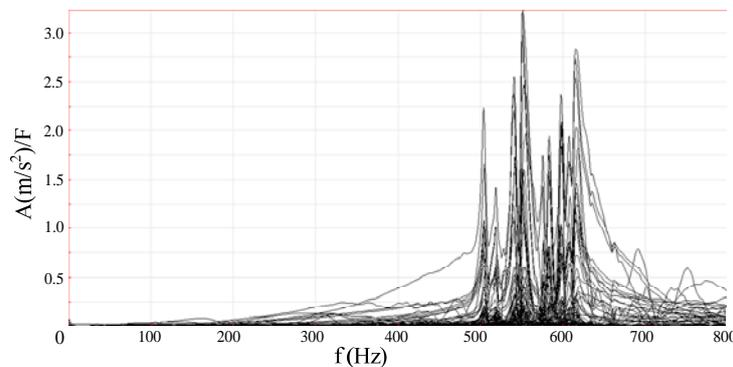
Figure 7. Response frequency curve of the guide
