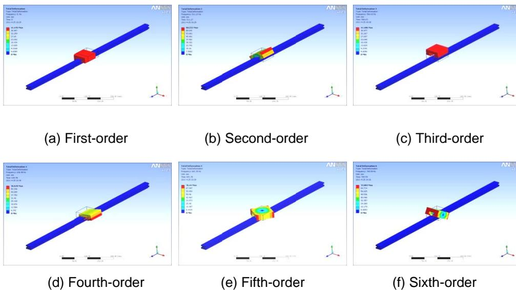
Figure 2. The first 6-order vibration modes on boundary condition 1
