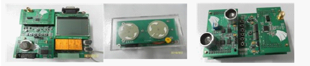
Figure 3. The coordinator node Figure 4. The DC motor node Figure 5. The Ultrasonic Sensor
