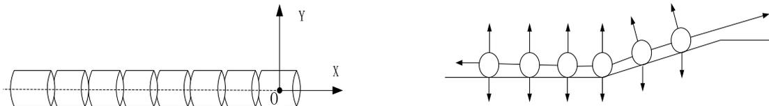
Figure 3. The coordinate relation between each train unit Figure 4. The multiple particles model
