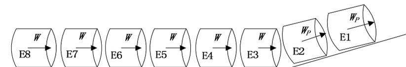
Figure 5. The force analysis of the multiple single-particle chain model
