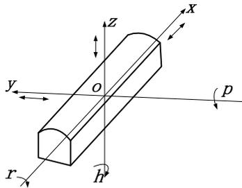
Figure 1 the local coordinate system of train
