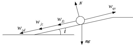
Figure 2 the single particle model of train
