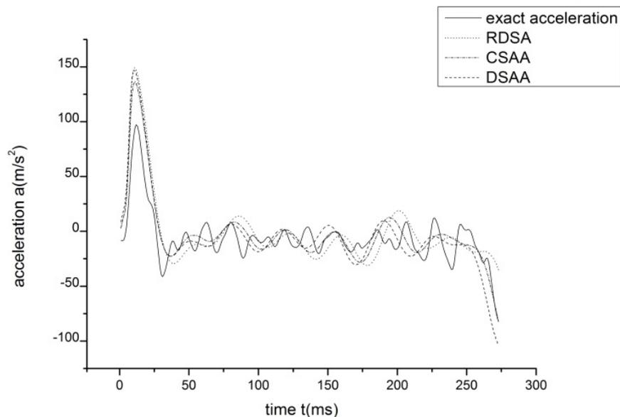
Figure 5. Actual Acceleration and Theory Acceleration Comparison
