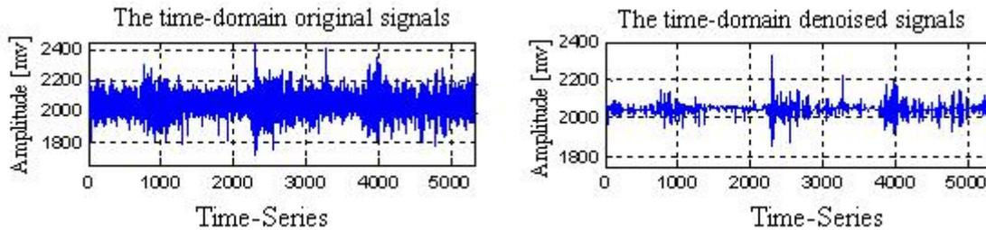
Figure 4. Time-domain graph before and after de-noising
