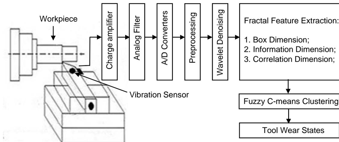
Figure 1. The block diagram of tool wear monitoring system
