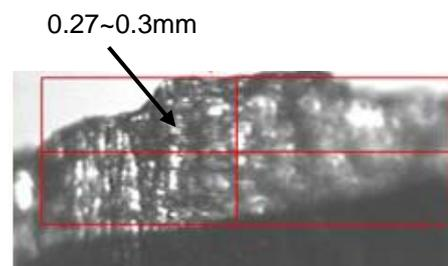
Figure 3. The picture of tool wear
