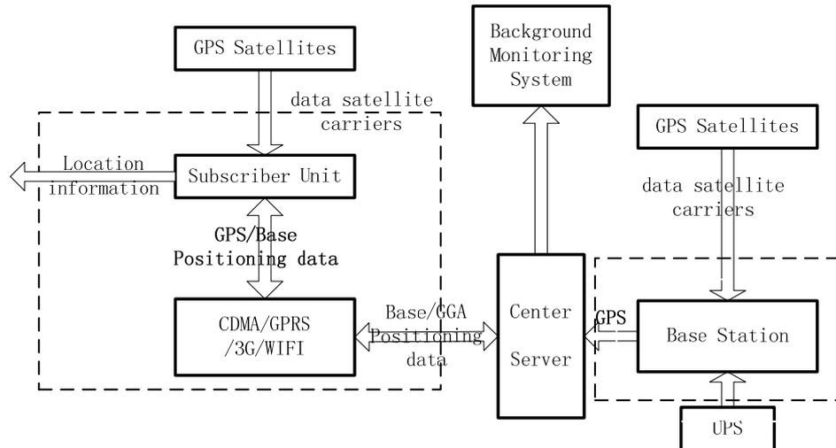
Figure 2. The system hardware diagram
