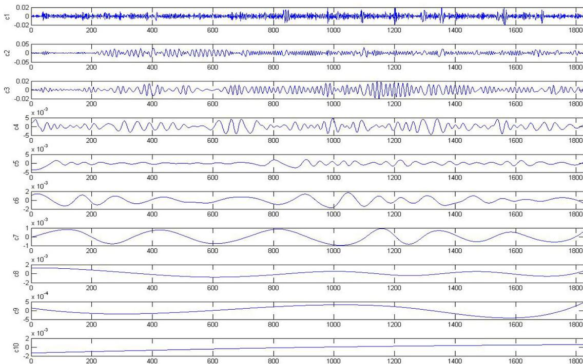
Figure 4. Decomposition of heave acceleration signal by EMD
