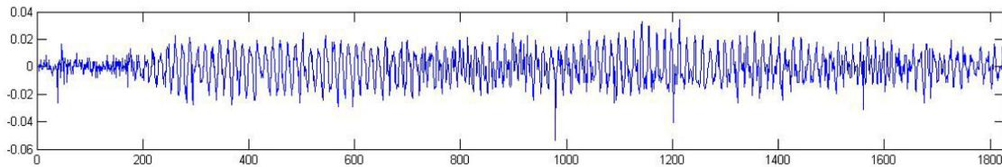
Figure 3. Original measured heave acceleration signal
