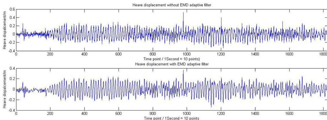
Figure 6. Integration of Heave acceleration with and without EMD adaptive filter
