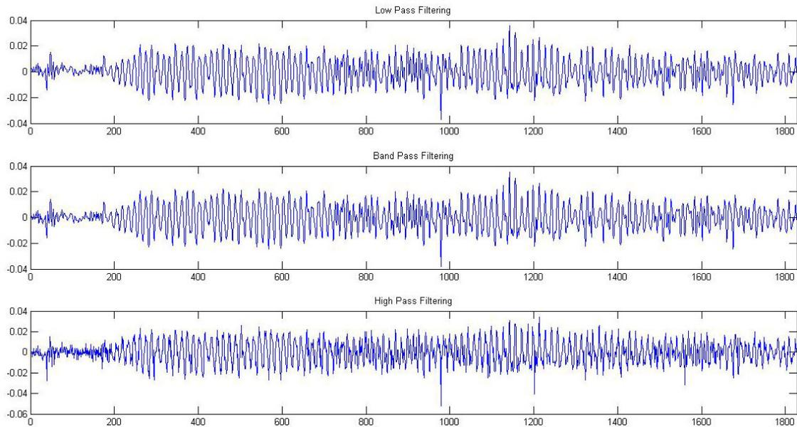
Figure 5. Reconstructed heave acceleration signal after EMD adaptive filtering
