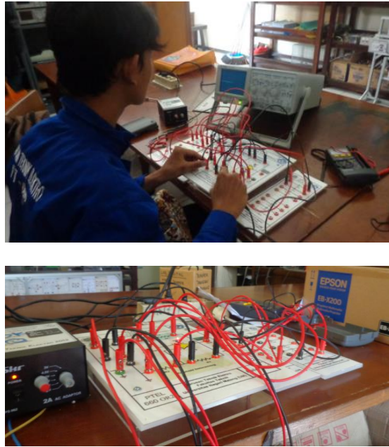
Figure 10. Testing the LC-Oscillator in Basic Electronic Laboratory State University of Malang (UM), Indonesia
