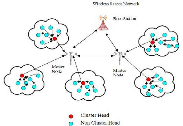
Figure 15. Clustered Wireless sensor network
