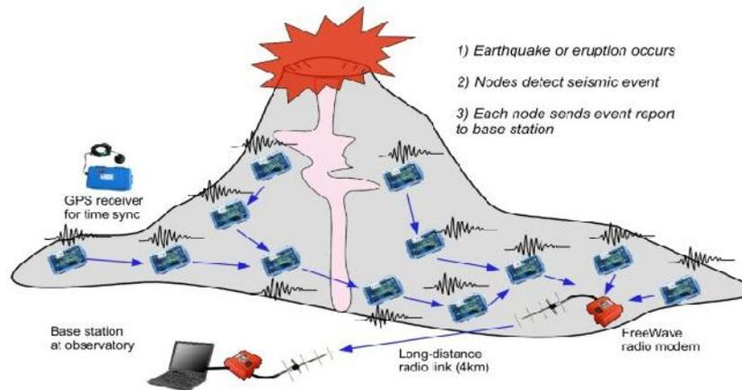
Figure 1. Example Wireless Sensor Network
