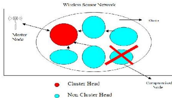
Figure 18. Compromised node deactivation and removal
