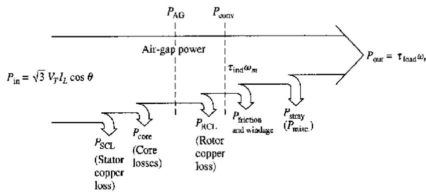
Figure 2. Power flow diagram of the induction motor
