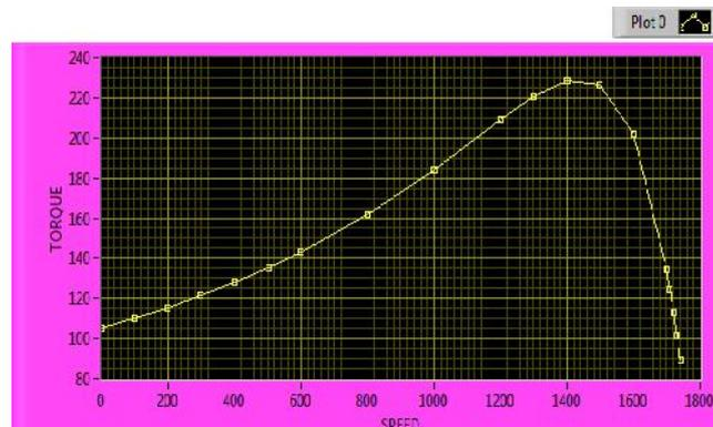
Figure 3. Torque vs Speed characteristics of induction motor
