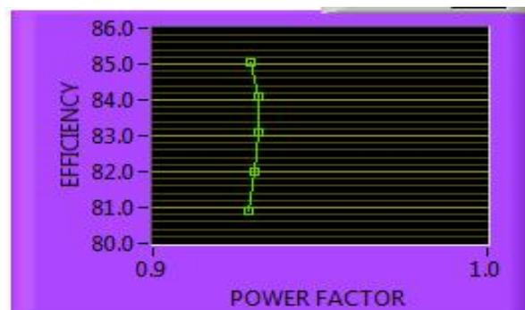
Figure 8. Power factor vs Efficiency characteristics of induction motor
