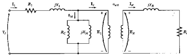
Figure 1. Equivalent Circuit Parameters of an Induction Motor
