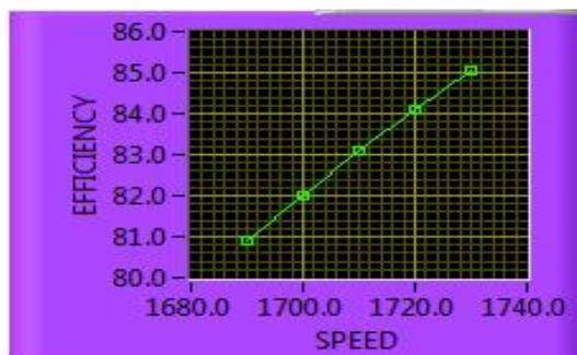
Figure 9. Speed vs Efficiency characteristics of induction motor
