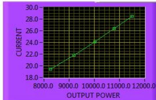
Figure 7. Output power vs Current characteristics of induction motor
