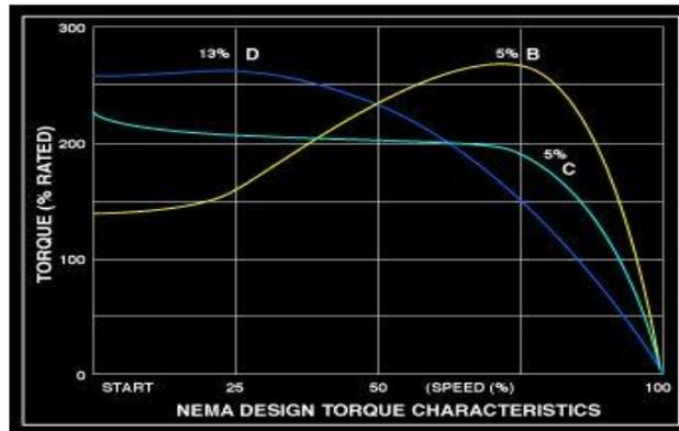
Figure 4. NEMA design Characteristics
