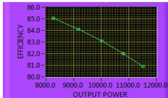
Figure 5. Output power vs Efficiency characteristics of induction motor
