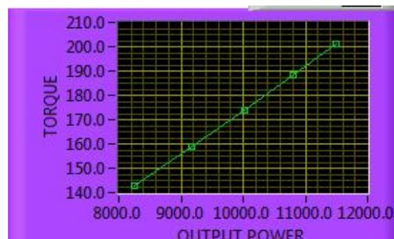
Figure 6. Output power vs Torque characteristics of induction motor
