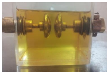
Figure 2. Spherical electrode with 2.5mm gap immersed with vegetable oil
