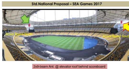
Figure 3. RF Antenna Proposed Location in Stadium
