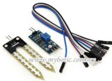
Figure 4. Soil Moisture Sensor
