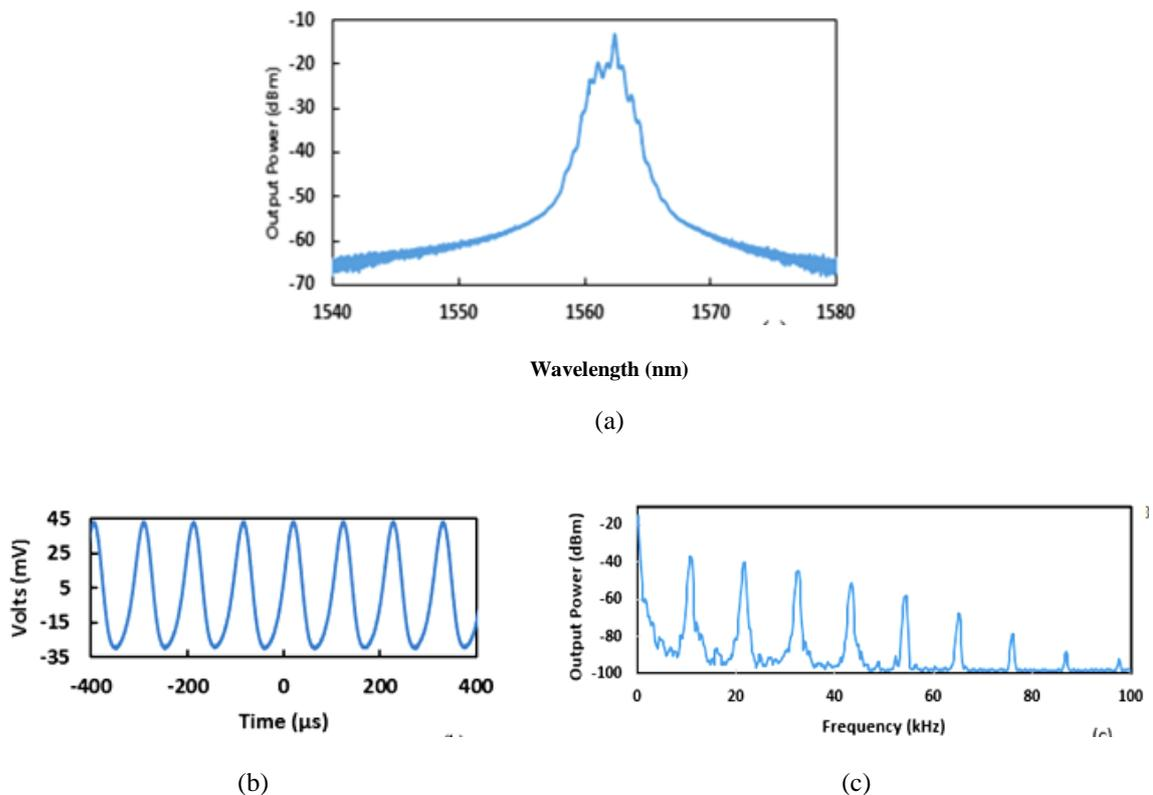
Figure 3. (a) Output Spectrum at 1562 nm Wavelength, (b) Pulse Period of 40.1  $\mu$ s, (c) RF Spectrum of the Output Power at SNR of 51dB
