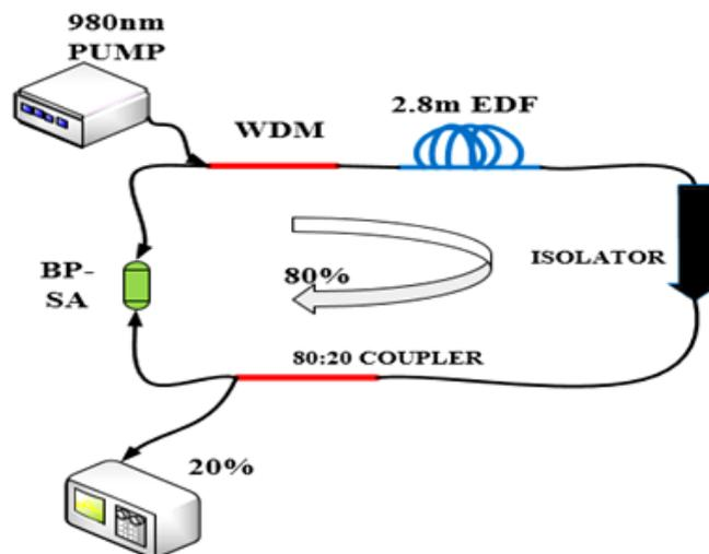
Figure 1. Configuration of Q-switched Setup
