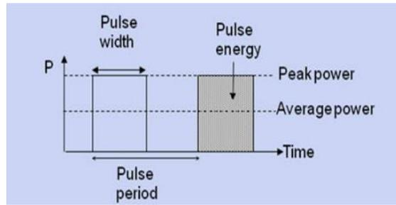
Figure 2. Relation between the Power and the Time
