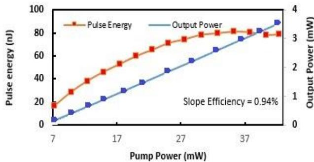
Figure 5. Output Power and Pulse Energy of Q-Switched Pulse versus the Pump Power
