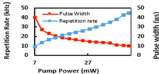
Figure 4. The Repletion Rate and Pulse width of the Proposed Q-Switched Fiber Laser.
