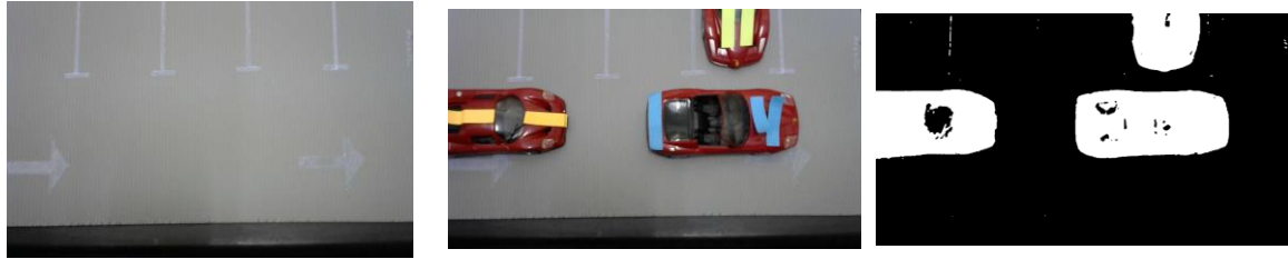
Figure 3. Sample image of (a)Background model, (b)Original image, (c)Foreground model
