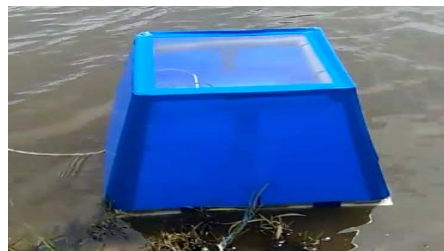
Figure 6. Smart Monitoring Water Quality Detector System
