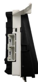
(b) Side view consists of two male connectors receiving frequency and resistance-based signals
