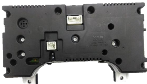
(a) Back view consists of two separated male connectors receiving +5 V, +12 V and ground signals
