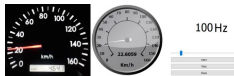
Figure 11. GUI and DUT corresponding speedometer reading for frequency generation of 100 Hz
