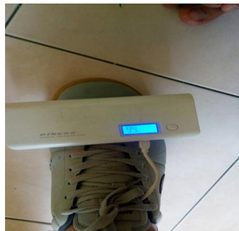
Figure 4. Prototype of piezoelectric shoe with external power storage
