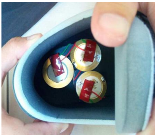
Figure 3. Prototype of piezoelectric shoe
