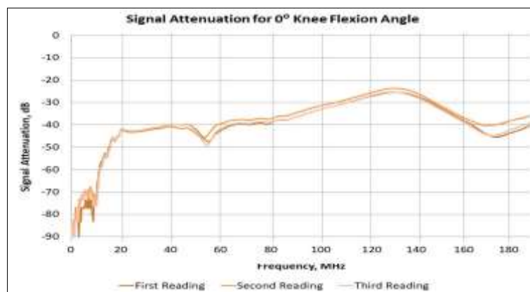
Figure 6. Signal Attenuation Captured at 0^\circ Knee Flexion Angle (No Knee Joint Existence)
