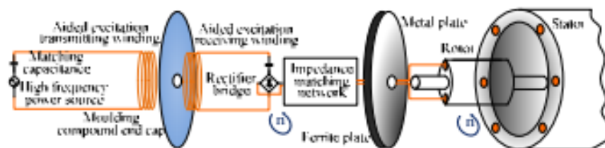
Figure 1. Structure of the brushless excitation mechanism
