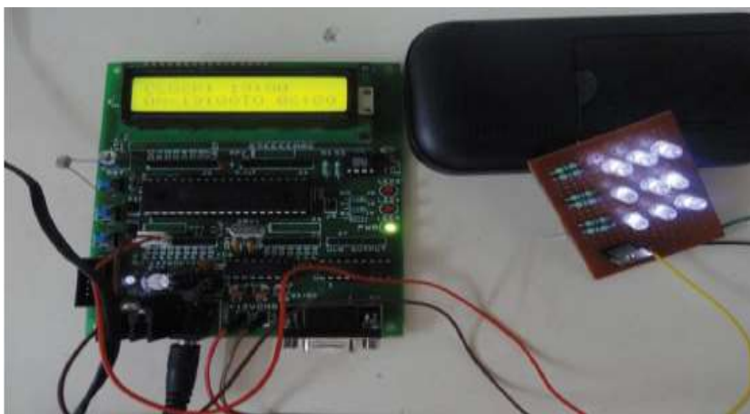
Figure 3. Prototype of Proposed Street Light System
