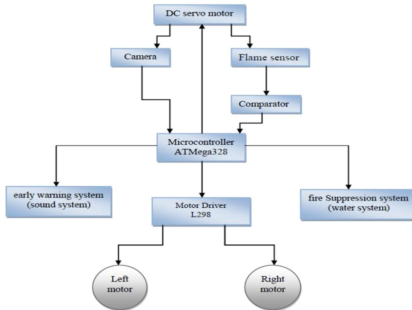
Figure 1. Block diagram
