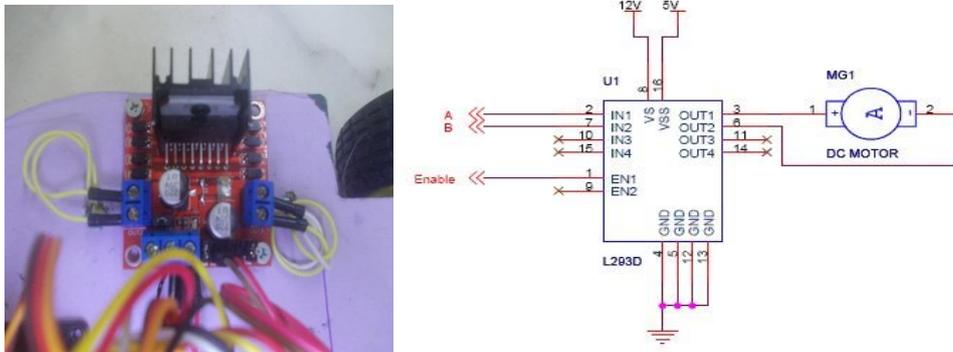
Figure 7. Driver L293 and schema
