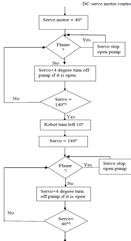
Figure 12. DC servo motor algorithm
