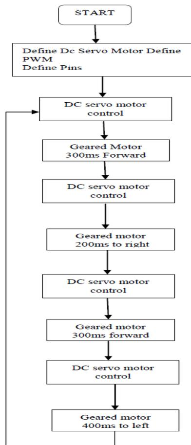
Figure 11. Fire tracking and suppression mobile robot algorithm
