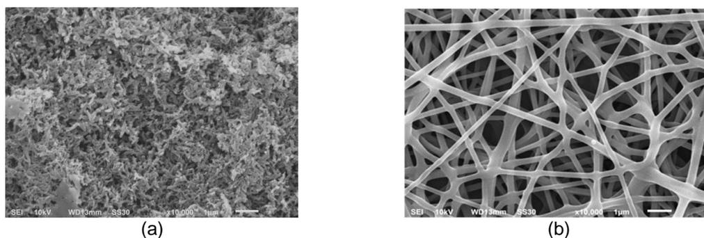
Figure 4. Structure of Polyaniline Fiber: (a) Result of interfacial polymerization, (b) Result of Electrospinning
