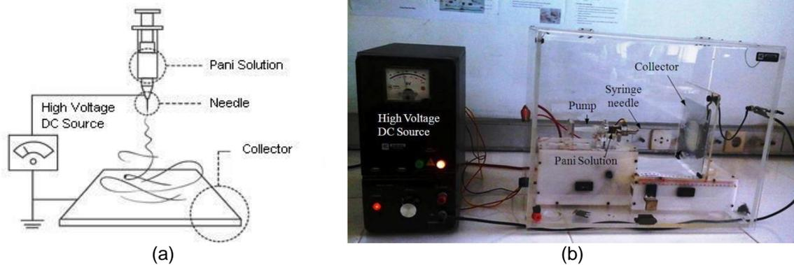
Figure 2. (a) Electrospinning Mechanism (b) Laboratory set up for electrospinning
