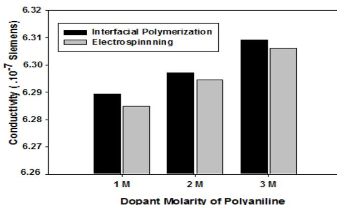
Figure 3. DC Electrical Conductivity of Polyaniline
