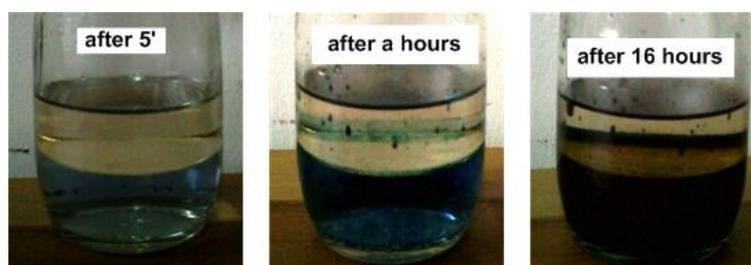
Figure 1. Polymerization Interfacial Process. The condition of solution after mixed the organic phase and the aqueous phase
