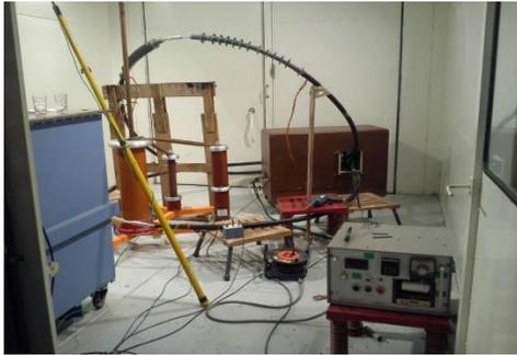
Figure 6a. Partial Discharge Measurement Circuit
